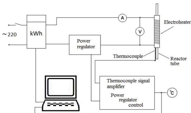
Figure 2. Scheme of heater power supply, measurement and adjustment of power consumption and temperature.
