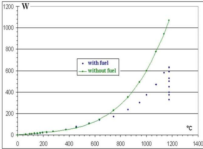
Figure 8. Power necessary for maintaining the set temperature.
