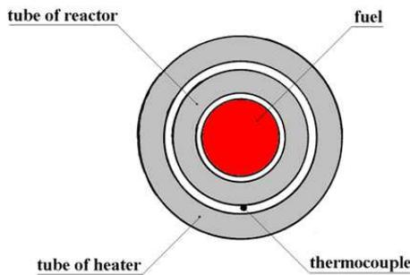
Figure 9. Cross-section of the reactor's central zone.
