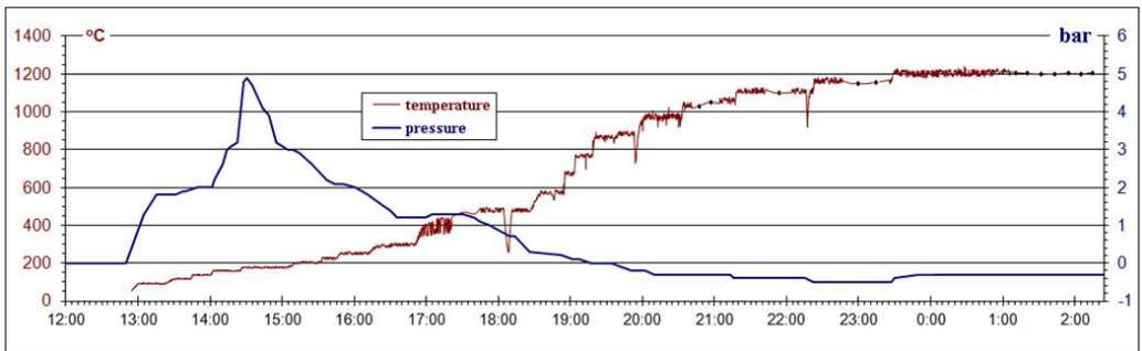
Figure 5. Heating the reactor to a working temperature. Change of pressure during the heating.
