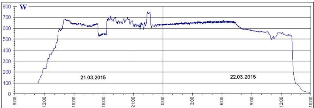
Figure 7. The power consumed by the reactor after it was switched on with a new heater. After achieving the temperature of 1200°C at 13:50 on 21.03.2015 this temperature was supported until 13:00 on 22.03.2015 by automatic adjustment of heater power.
