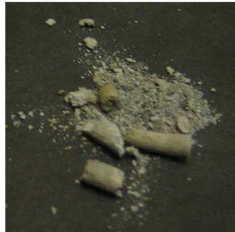
Figure 11. Fuel after extraction from the container.
