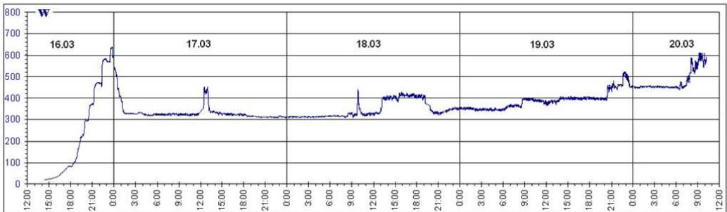
Figure 6. The power of heating during almost 4 days until the heater is burned out. After achieving the temperature of 1200°C at 23:30 on 16.03.2015 this temperature was maintained until 10:50 on 20.03.2015 by automatic adjustment of heater power.
