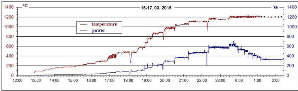
Figure 4. Heating the reactor to a working temperature. The Moscow time (UT+3) is shown on the horizontal scale.
