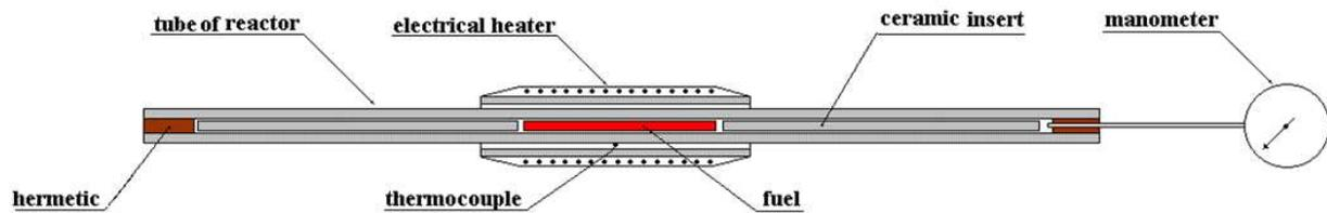
Figure 1. Structure of the reactor designed for a long-term operation.
